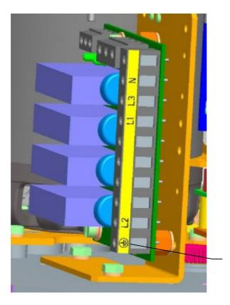
INTERNAL PROTECTION TERMINAL FOR THREE PHASE VERSION WITH SSR
