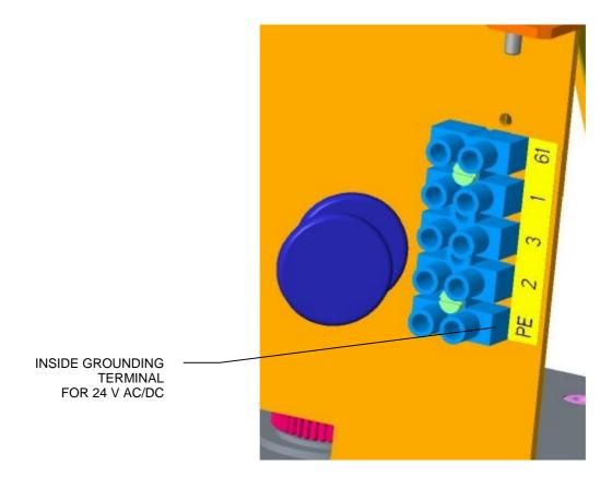
Fig. 2h- Supply terminals and PE for AE SPR 2.XPA
