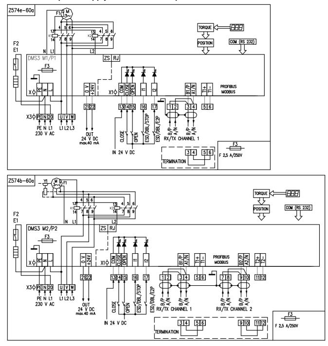
Wiring diagrams of EA SPR 1PA with DMS3 electronic control with Modbus/Profibus protocol for three - phase supply – for ambient temperature -60°C to +40°
