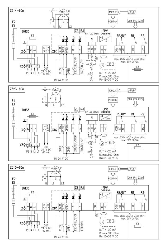
Wiring diagrams EA SPR PA– single - phase supply – for ambient temperature -60°C do +40°
