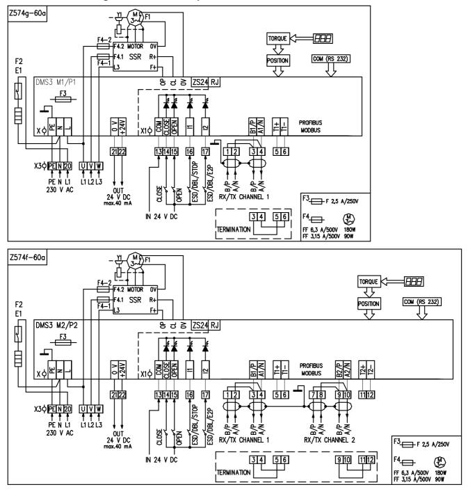
Wiring diagrams EA SPR 2.XPA with Modbus/Profibus protocol – for three phase supply, withcontactless switching – for ambient temperature -60°C to +40
