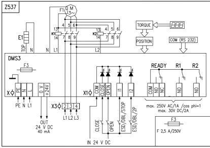
Wiring diagrams EA SPR 2.XPA – for three - phase supply, reserve contactors
