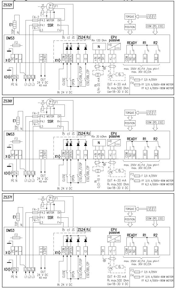
Wiring diagrams EA SPR 2.XPA – for three phase supply with-contactless switching
