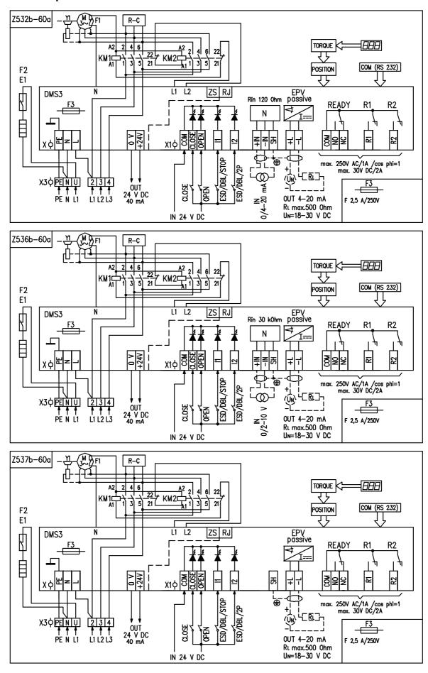
Wiring diagrams EA SPR 2.XPA – three - phase supply, reserve contactors – for ambient temperature -60°C do +40°
