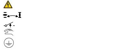
Dangerous voltage (EN ISO 7010-W012) Stroke of the electric part-turn actuator Switching-off torque Manual control (0096 ISO 7000) Protection terminal (5019 IEC 60417)
