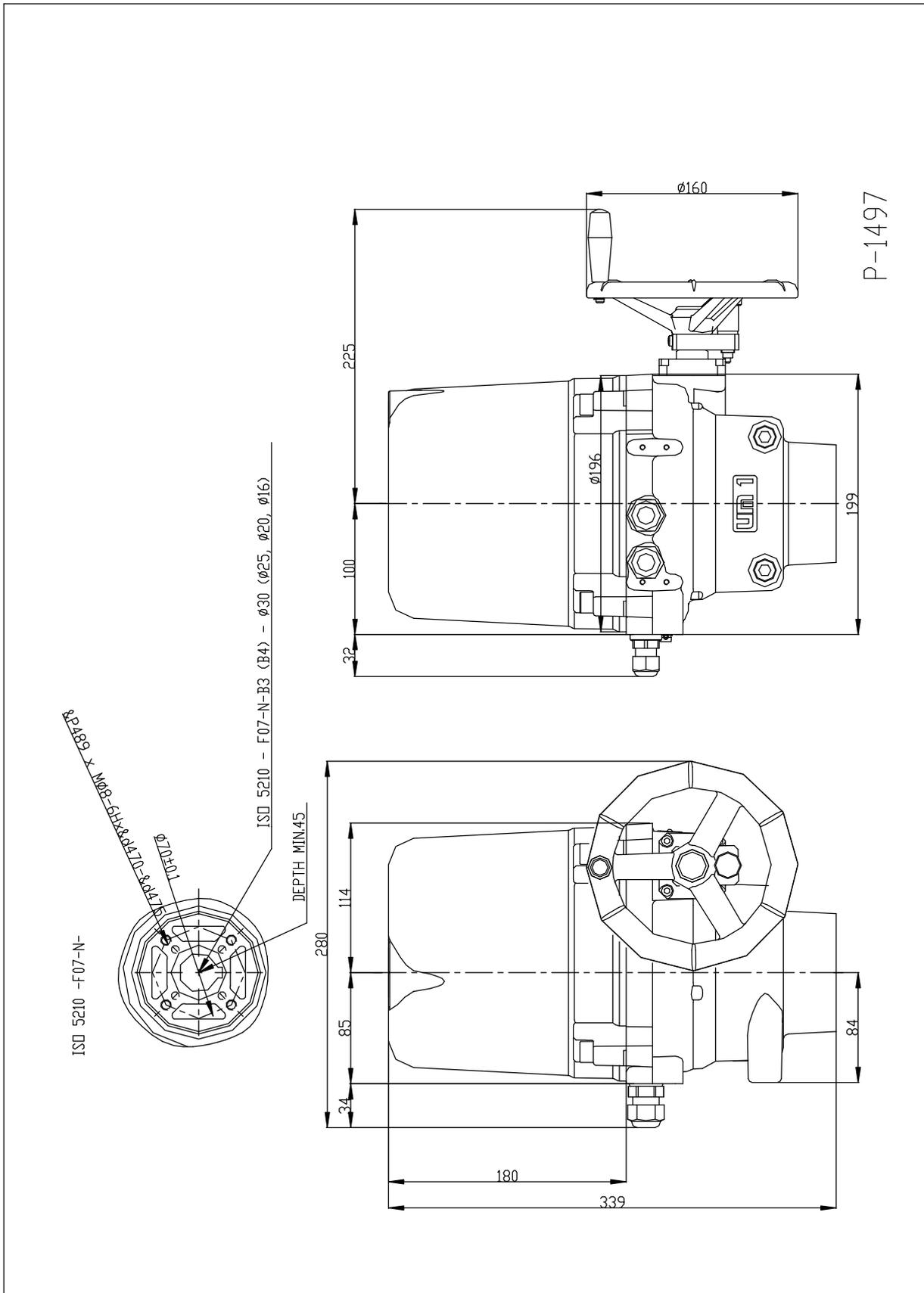
Explosion-proof electric multi-turn actuators Unimact **UM 1-Ex** – flange connection DIN 3338
