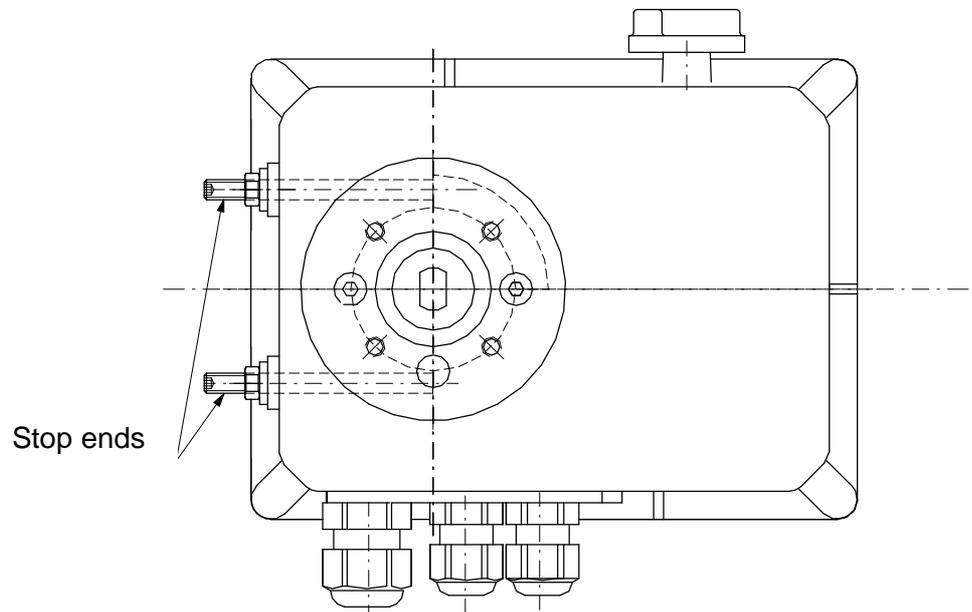
Pic.9: Flange of actuator from bottom.
