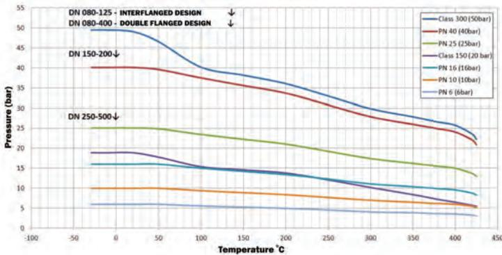
Pressure and temperature curve
