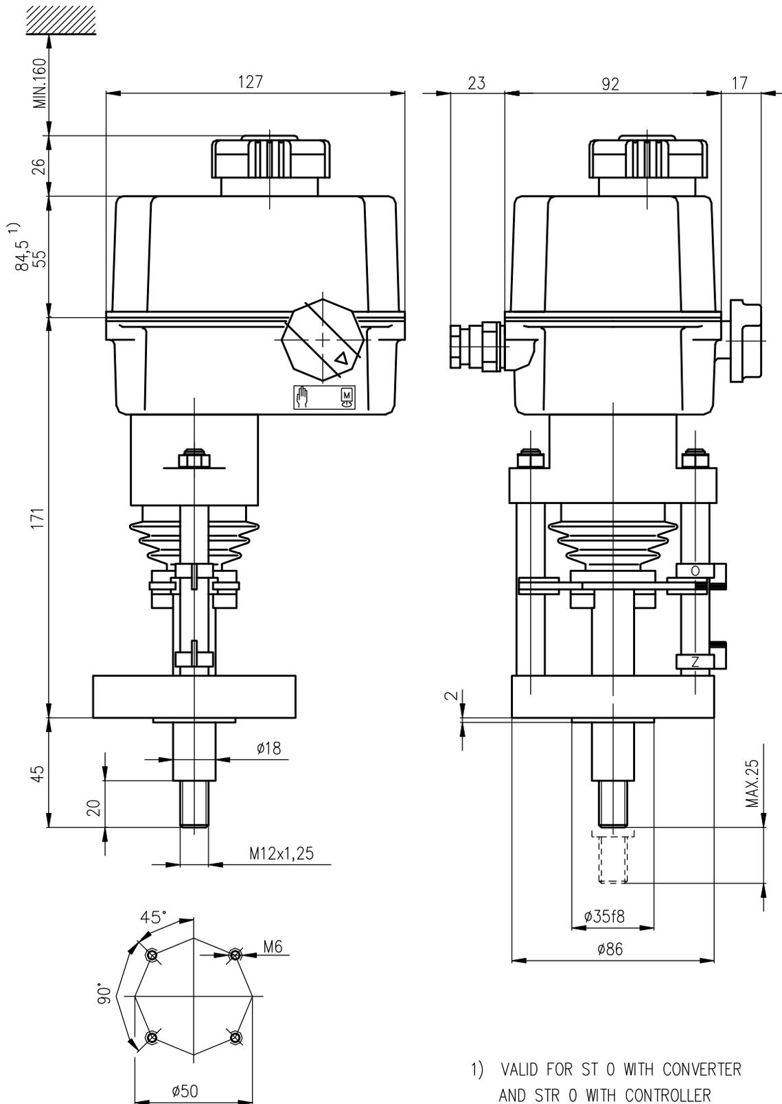
1) VALID FOR ST 0 WITH CONVERTER AND STR 0 WITH CONTROLLER
